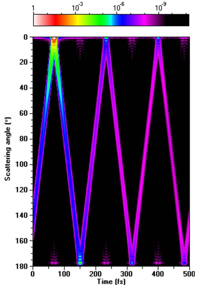
Fig. 5. (Color online) Diffracted intensity corresponding to Eq. (4) as a function of the scattering angle and delay time for the unpolarized raised cosine pulse of [29] with  $\lambda_0 = 0.65 \mu\text{m}$  and  $\tau = 10 \text{ fs}$  incident on a spherical particle of radius  $a = 8 \mu\text{m}$  and refractive index  $N + iK = 1.3326 + i(1.67 \times 10^{-8})$ .
