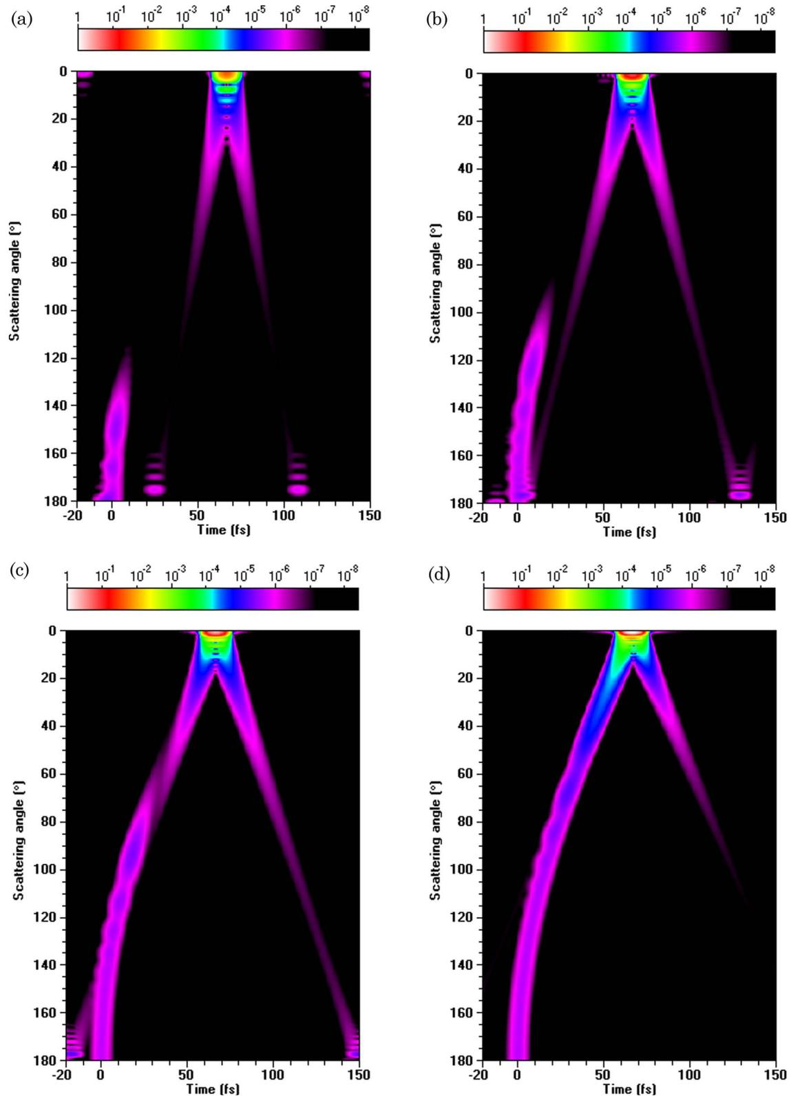
Fig. 6. (Color online) Intensity of the  $p = 0$  Mie-Debye term as a function of the scattering angle and delay time for the unpolarized raised cosine pulse of Fig. 5 incident on the spherical particle of Fig. 1. The upper limit of the Mie sum is (a)  $0.4ka$ , (b)  $0.6ka$ , (c)  $0.8ka$ , and (d)  $1.0ka$ .
