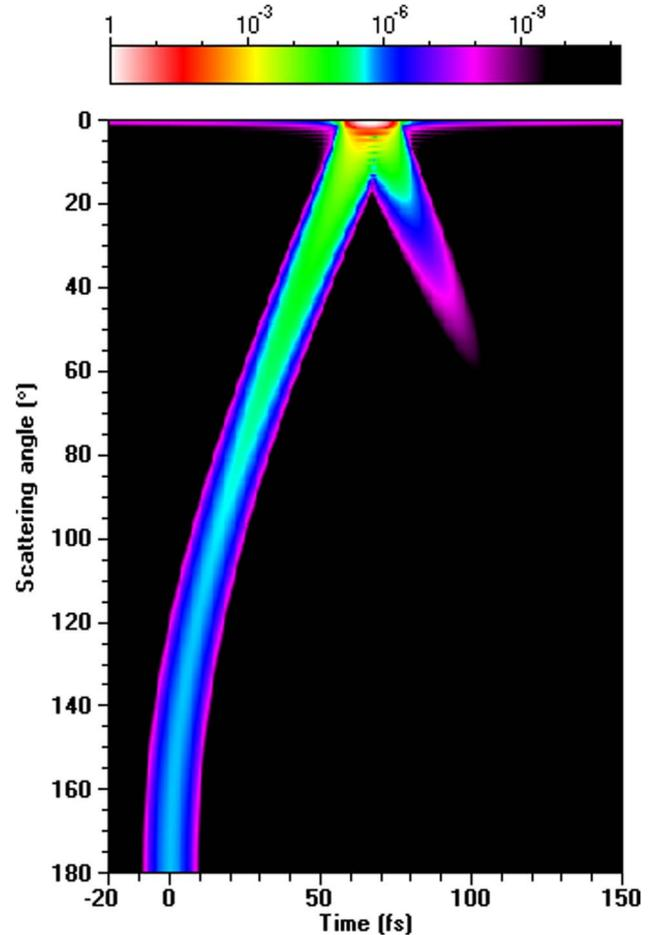
Fig. 1. (Color online) Intensity of the  $p = 0$  Mie–Debye term as a function of the scattering angle and delay time for the unpolarized raised cosine pulse of [29] with  $\lambda_0 = 0.65 \mu\text{m}$ , and  $\tau = 5$  fs incident on a spherical particle of radius  $a = 10 \mu\text{m}$  and refractive index  $N + iK = 1.3326 + i(1.67 \times 10^{-8})$ .
