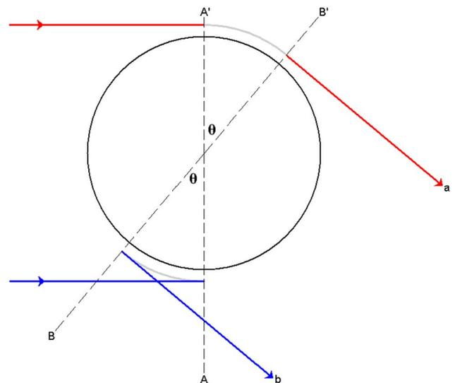
Fig. 2. (Color online) Diffracted rays a and b are assumed to arrive at the entrance plane A'A with the same phase. Then ray a advances its phase by  $ka\theta(1+1/ka)$  between the entrance plane and the exit plane B'B for scattering at the angle  $\theta$ . The diffracted ray b retards its phase by  $ka\theta(1+1/ka)$  between the entrance and exit planes.
