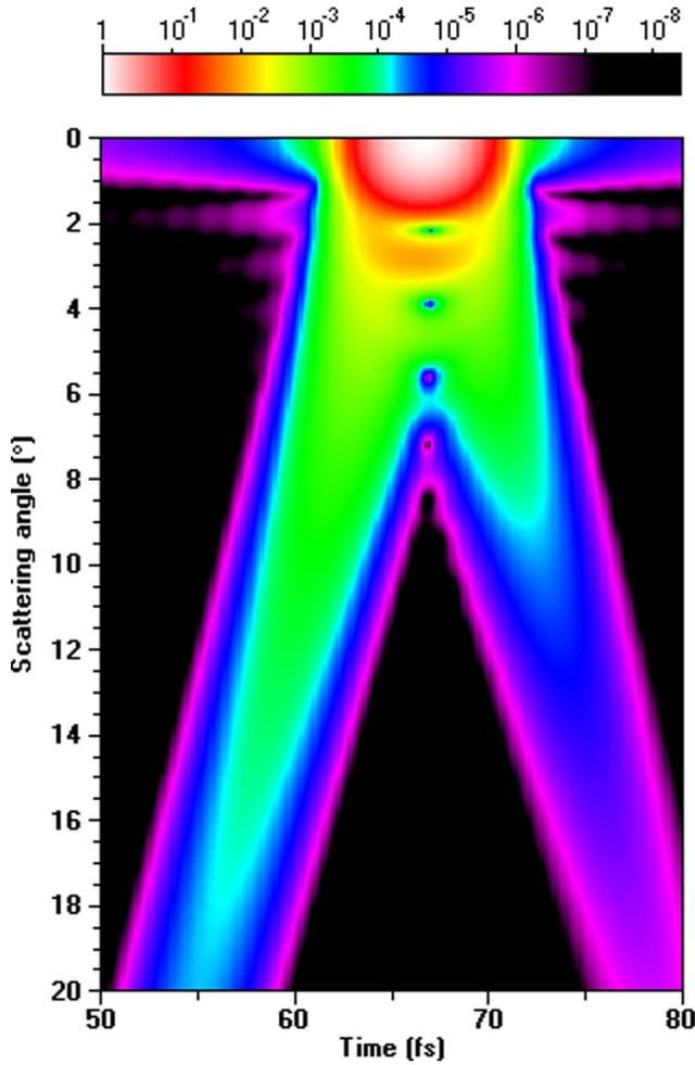
Fig. 4. (Color online) Intensity of the  $p = 0$  Mie–Debye term as a function of scattering angle and delay time in the near-forward direction for the unpolarized raised cosine pulse and spherical particle of Fig. 1. The fundamental sampling interval is 0.135 fs.
